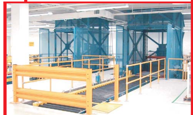
Continuous Vertical Lifts with 6,000 lbs. capacity, used to transport materials and finished product by pallet from the ground to the third floor and vice versa.
