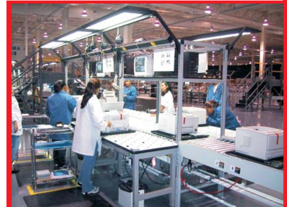
Workstations integrated into conveyor system.
