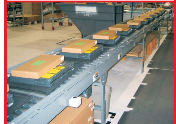
Motorized Roller Conveyor allows tracking and total control of product, ensuring no contact between valuable units.
